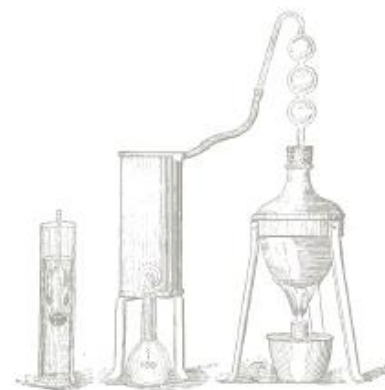
FIG. 18.—German Laboratory Apparatus for the Estimation of Alcohol in the Wash Liquor.
